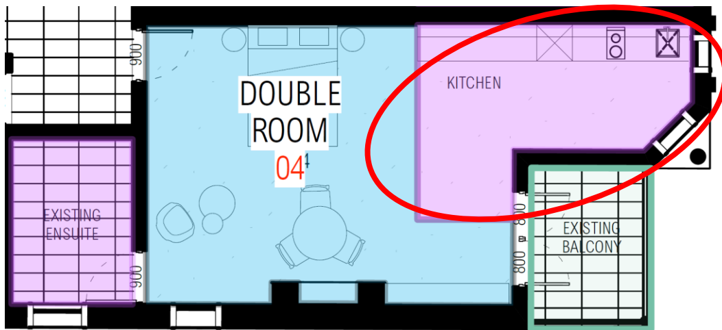
Figure 43: Plan area calculation sheet extract depicting boarding room 04, with the excessive kitchen size circled in red
